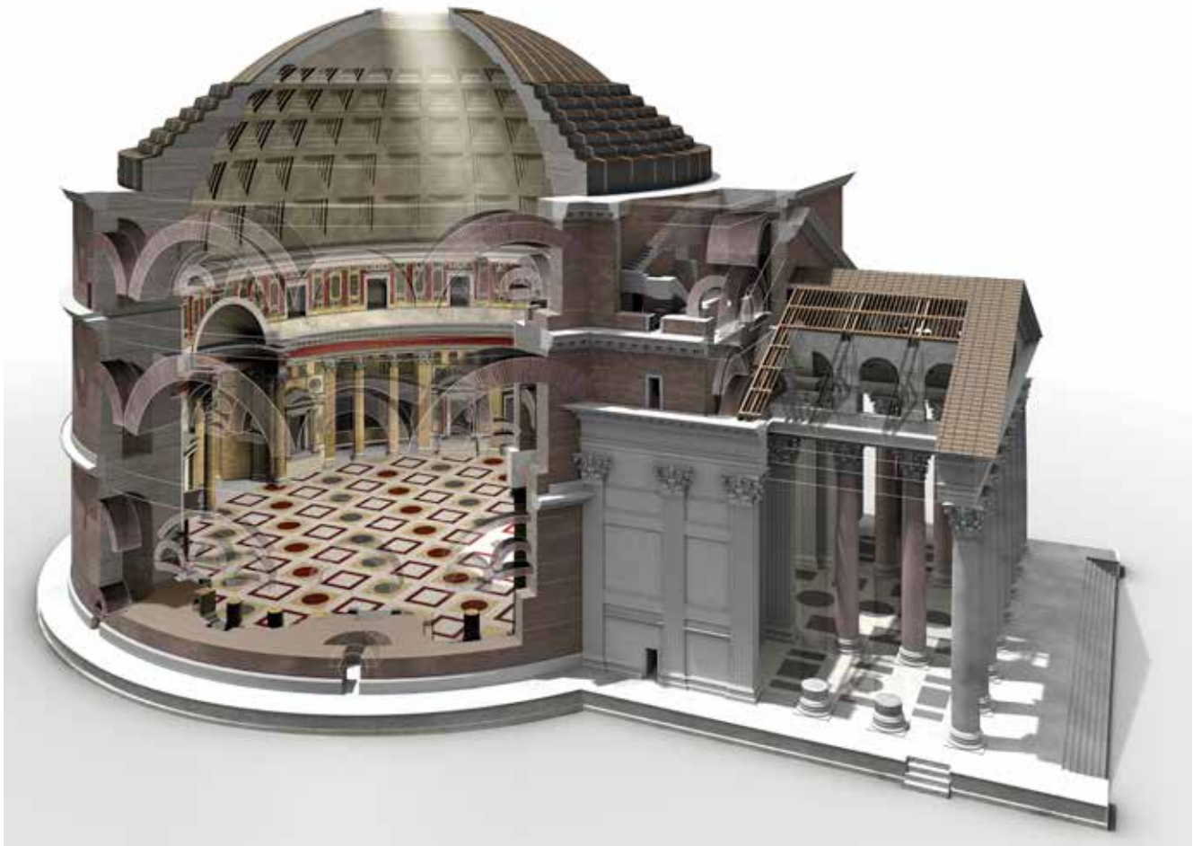
Plate 1 Cut-away of three-dimensional virtual model of the Pantheon (conceived by the author, created by Robert Grover)
