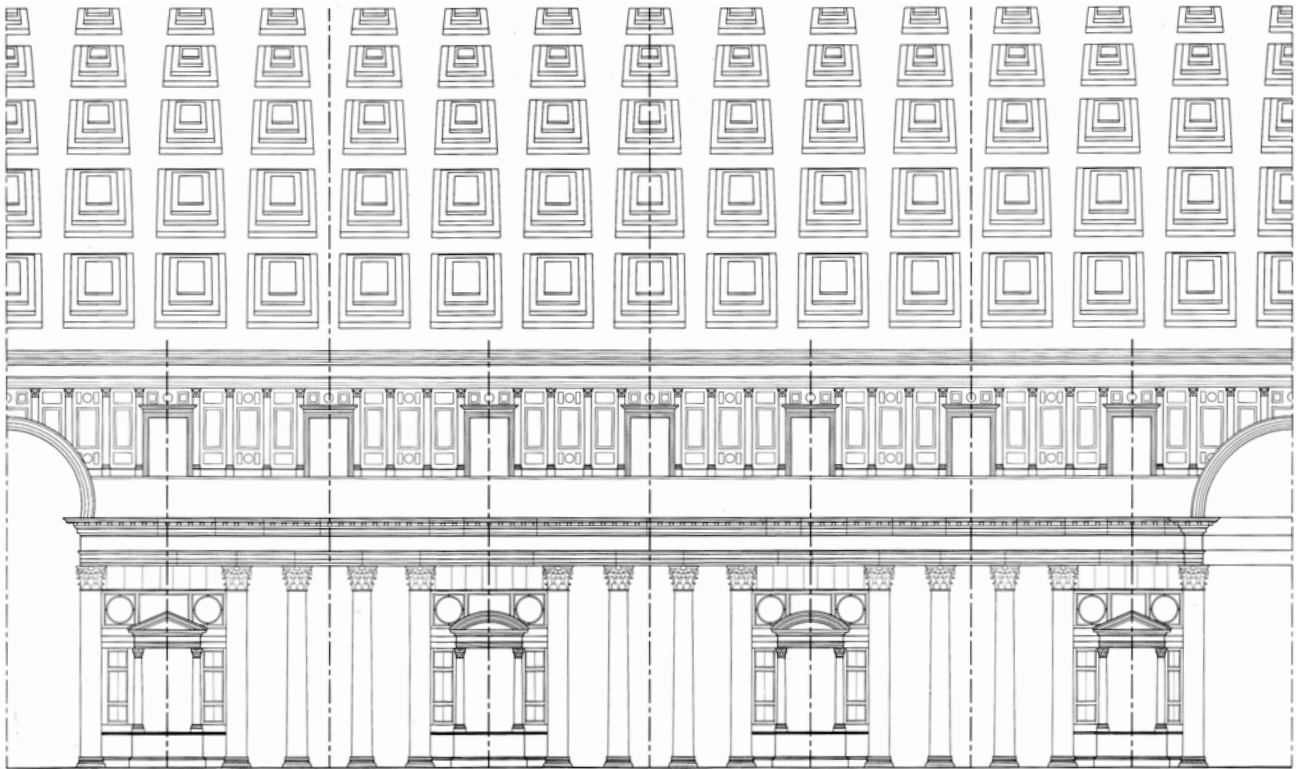
Plate 6 Pantheon, interior elevation of the rotunda projected flat. The only instances in which there is concordance between different levels of the composition are indicated by dotted lines (author: from Wilson Jones 2000, fig. 9.25)
